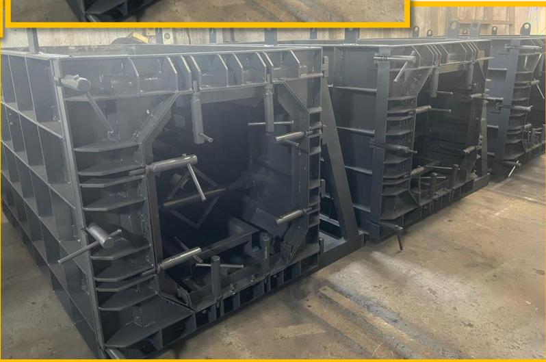
**L & T - NATIONAL RAIL HIGH SPEED NOISE BARRIER (BULLET TRAIN) HYDRAULIC MOULD**
